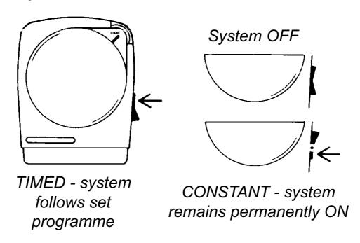
The 103 unit is now set, and the current status of the timeswitch can be seen on the wheel at the top righthand corner of the unit, (e.g. "OFF UNTIL C").
