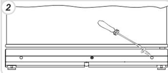
3 Drill the plinth on the marked left hand-side area.
