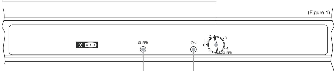
The orange light comes on when the thermostat knob is turned to SUPER. In this case the compressor continues to function as normal.
